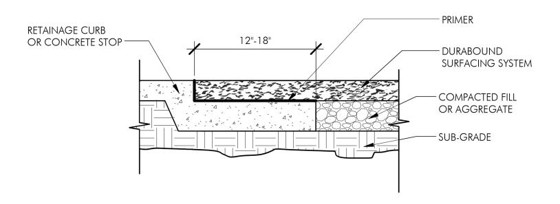
DURABOUND SURFACING SYSTEMS: COMPACTED STONE WITH CURB DETAIL (MUST HAVE EXCELLENT DRAINAGE)
